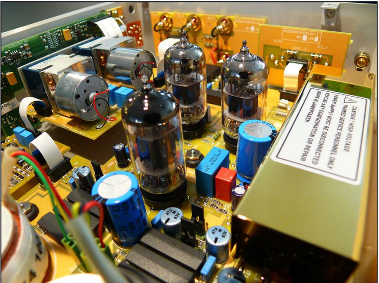
The volume and balance pots are made by Alps to Nagra's specifications.
