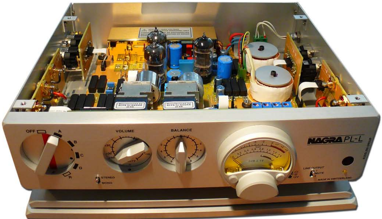
Here we have the vacuum-tube PL-L version of Nagra's preamps sans phono module and top panel.
